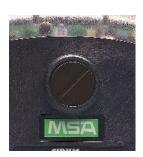
PID lamp access is made easy with the Sirius unit. When users need to change or clean a PID lamp, it is so simple with a twist of the lamp holder located conveniently on the front of the instrument. Color-coded lamp eV
