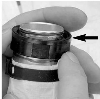
2. Check the end of the hood coupling nut for an O-ring.
