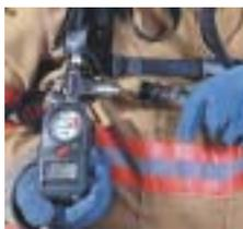
The patented **Quick-Fill® System** lets MSA Air Mask users refill and transfill air cylinders without removing their mask or air cylinder. They can 1) fill an SCBA cylinder from a mobile compressor or cascade system in less than a minute; 2) transfill
