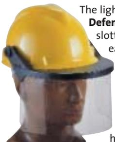
The lightweight polypropylene **Defender® Faceshield Frame** for slotted caps features easy-in, easy-out visor replacement; front drop-edge splash protection; lockdown clip; unlimited lift positions; long-lasting O-ring pivot-joint design; and a snap-in ear muff option. No hardhat is required for the Defender Headgear Faceshield Frame with SparkGard™ Faceshield and ratchet suspension.
