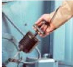
MSA's **Toximeter™ II Automatic Pump** allows the user to preset the number of pump strokes (from 1 to 250). Intrinsically safe, it works with all MSA detector tubes and can also be used as a sampling pump.
