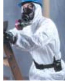
MSA's low-profile **OptimAir® MM 2K PAPR** consists of a mask-mounted motor/blower with HEPA filter for particulates and a small water-resistant NiMH battery pack, plus full facepiece, belt, and cable. Its dual-rate battery charger recharges the battery in less than 3 hours. Benefits include extremely light weight, easy maneuverability and decontamination, and 8 hours of battery use.
