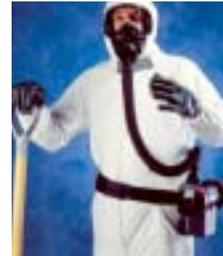
The **OptimAir® 6A PAPR** has a belt-mounted blower/motor with breathing tube to the full- or half-mask facepiece and a maintenance-free lithium battery. It is used with an entire family of filters and cartridges for protection against particulates and/or toxic gases and vapors. Optional equipment includes a Tyvek hood (with HEPA filters only) and a rechargeable NiCd battery.
