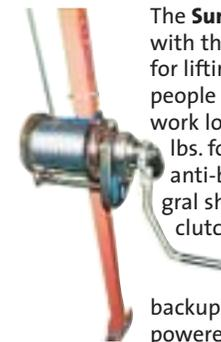
The **Sure-Strong™ Work Winch**, used with the Sure-Strong Tripod, is made for lifting, lowering, and positioning people and materials (maximum work load of 310 lbs. per person, 620 lbs. for materials). It features an anti-backlash crank handle, integral shock absorber, load-limiting clutch, emergency drive for manual bypass when necessary, two independent secondary backup brakes, and an optional air-powered drive assembly.
