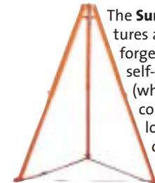
The **Sure-Strong™ Rescue Tripod** features adjustable aluminum legs; forged steel anchor eyes in the self-locking head assembly (which prevents unintentional collapse); legs that adjust and lock individually to accommodate variations in anchor heights, uneven ground, etc.; and leg security straps. It is rated for 2 people with a working load of 1,100 lbs.
