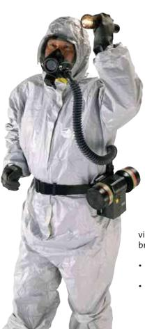
A powered air-purifying respirator that filters contaminants from ambient air via CBA/RCA OptiFilter® Cartridges. Beltmounted motor/blower provides constant air flow via breathing tube to facepiece.
