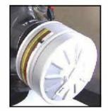
When accompanied with a face-piece (e.g., full mask), a respirator filter forms a filter apparatus. Filter apparatus sets are used to remove harmful gases, vapors and solid particles from inhaled air. The performance of this filter complies with EN 141, 143, and 371 as well as other regulations. Test certificates and qualifications are available for this respiratory filter on page 31.
